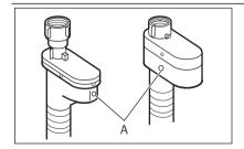
The inlet hose has a water stop device. This device prevents water leaks in the hose because of its natural ageing. The red sector in the window «A» shows this fault.
